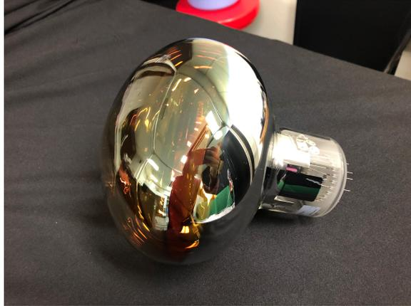
**Figure 3.3:** 8” Hamamatsu R5912-100-70 PMT. The yellow hemispherical surface is the photocathode made of bialkali and it is vacuum inside.
