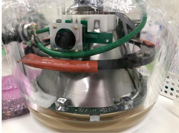
**Figure 5.11:** Cameras in a D-Egg.
