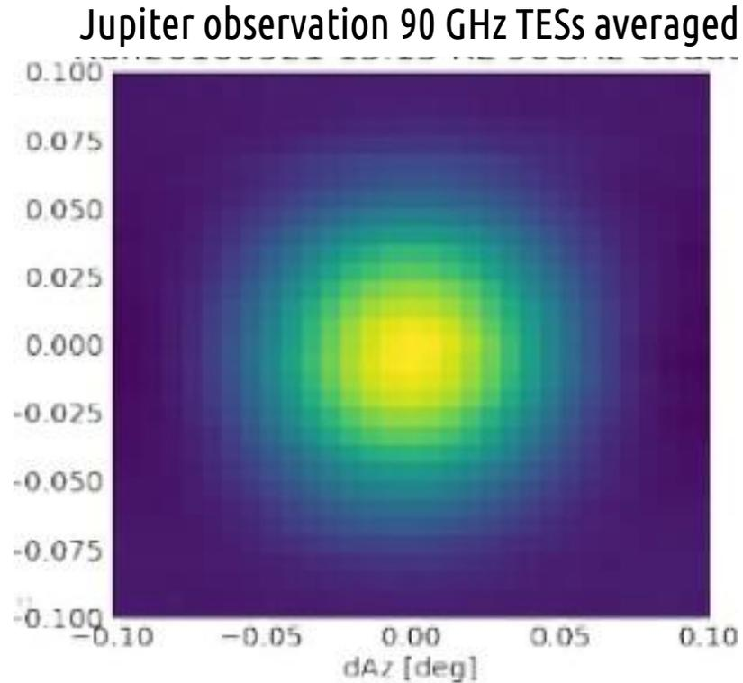
Telescope focusing performance is checked with planet observation.
