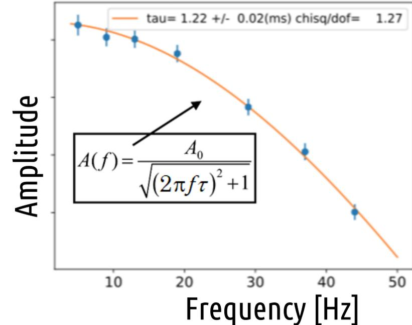
3. Fit curve to obtain gain and time constant of detector
