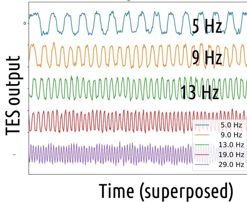
2. Measure detector output amplitude for each frequency
