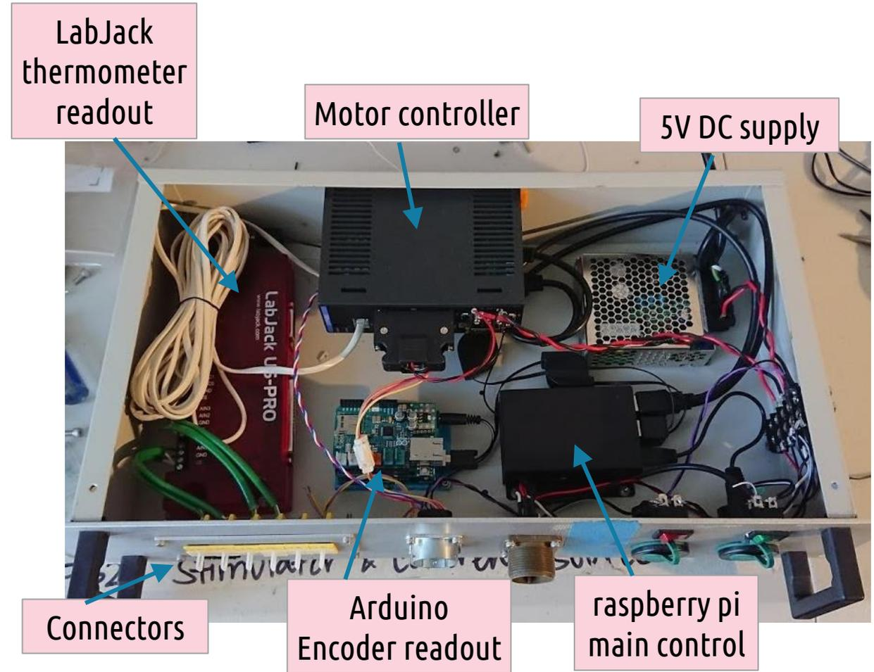
Controlling electronics are installed in a 19" box, and it is inserted in a telescope co-moving rack.
