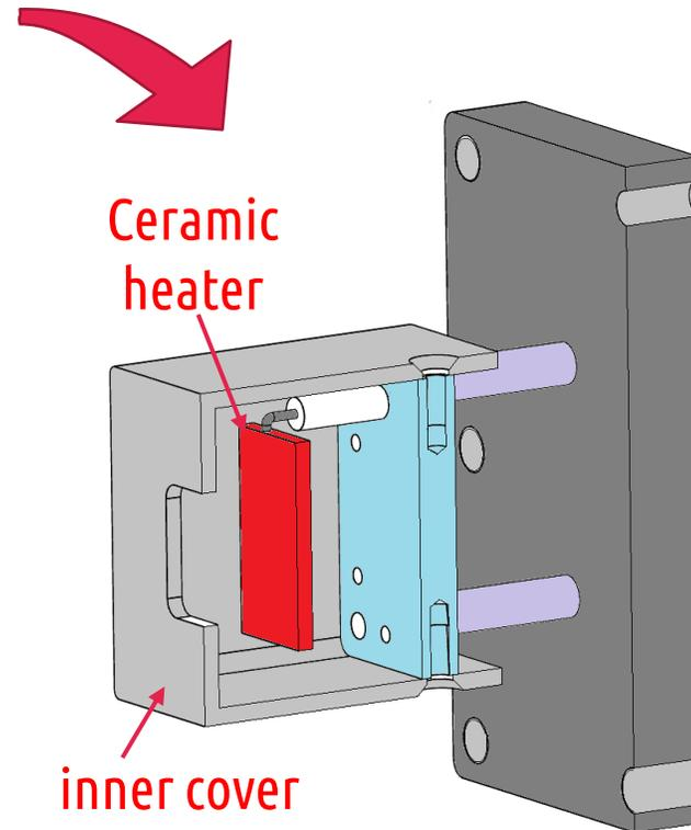
cross-section image of heater unit. Heater unit could be replaced on telescope with minimal cabling work.
