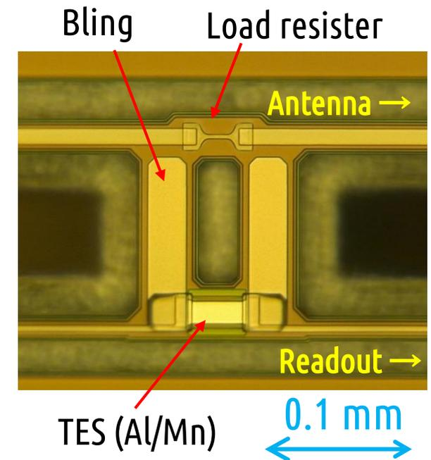
SA adopts frequency multiplexing, 40 channels are read with one SQUID
