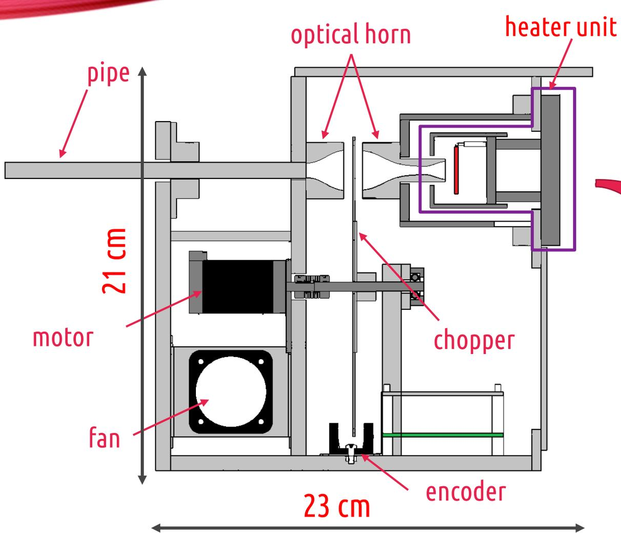
Black body radiation from ceramic heater ( $\sim 700^{\circ}\text{C}$ ) is modulated with chopper and is emitted from the pipe to the receiver.
